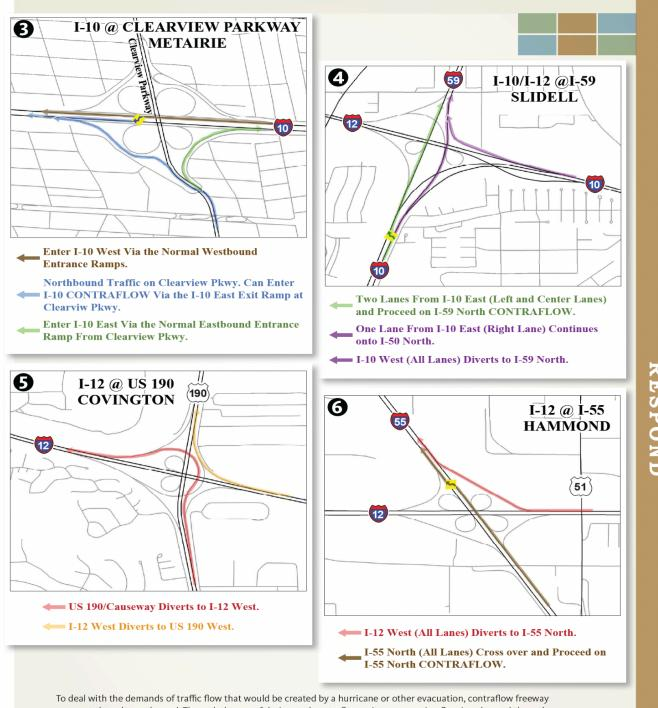
segments have been planned. Through the use of designated contraflow points, evacuation flow is enhanced through movement of all traffic in the same direction. This diversion enables some or all normally incoming lanes to serve as outgoing lanes to facilitate and speed evacuation. Several different routes and contraflow crossover points are planned for use in an evacuation of the Southeast Louisiana area.
