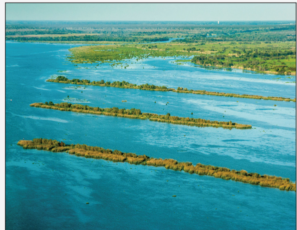
Cote Blanche Bay in Louisiana has artificial islands that were created to help protect the mainland.
