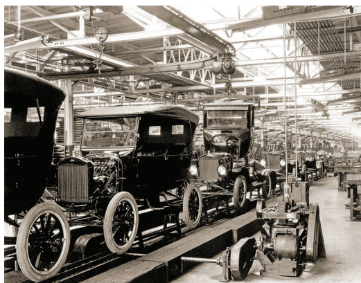
By the 1920s, Ford's assembly line had been adopted in mass production facilities across the country.
